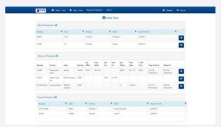
In addition, **SENSAP<sup>TM</sup> EDGE** server provides overall visualization of the shop-floor, by listing all production machines on one screen. This way, shop floor managers can be aware of each machine's status, as well as the progress of the job in production.
